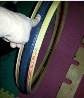
3. Install one side of the tire, beginning opposite the valve hole
